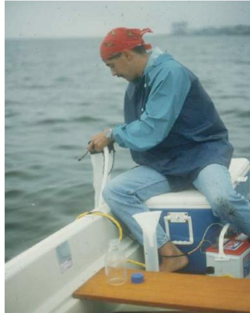
**Figure 4.** Mr. Joseph Goncalo demonstrating the method of using a submerged 12-V bilge pump to obtain water samples for analysis of larval bivalves in the water column. Note the presence of a 1-liter glass sample bottle containing a pre-measured volume of alcohol to kill and preserve the mussel larvae and all the other plankton in the water sample. Photo by Michael A. Rice, University of Rhode Island.
