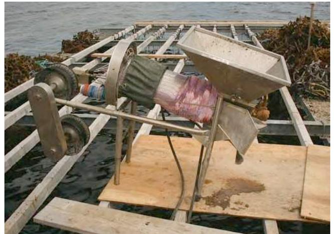
**Figure 7. Mussel socking machine, manufactured by Aguin, used in mussel raft culture. Drop lines are fed under the hopper, and mussels are wrapped up against the line by cotton sheeting. The cotton sheet degrades, after the mussels have attached their byssal threads to the dropline. Photo courtesy of Carter Newell, Pemaquid Mussel Farms.**
